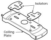
Figure 2a - Adding Isolators to Ceiling Plate
